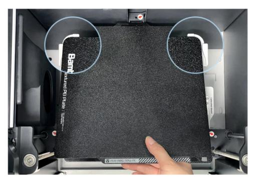
Step 1: Align the plate with the fixed points of the platform with the name of the plate facing you
