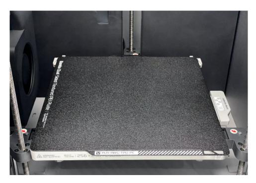
Step 2: Lower the plate and secure to the magnetic platform
