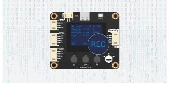
16M storage for storing data in real-time with accurate time tags, can store 400000 pieces of data.
