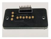
2) Attach 3 pin Headers to 3.3V,Vcc GND connection as shown and solder from Bottom.
